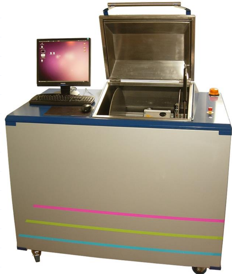
Assembled small animal micro-CT scanner
