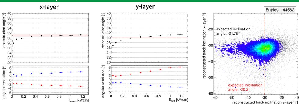
→ three-dimensional μTPC reconstruction with angular resolution of  $+3^\circ$   $-2^\circ$  in both layers
