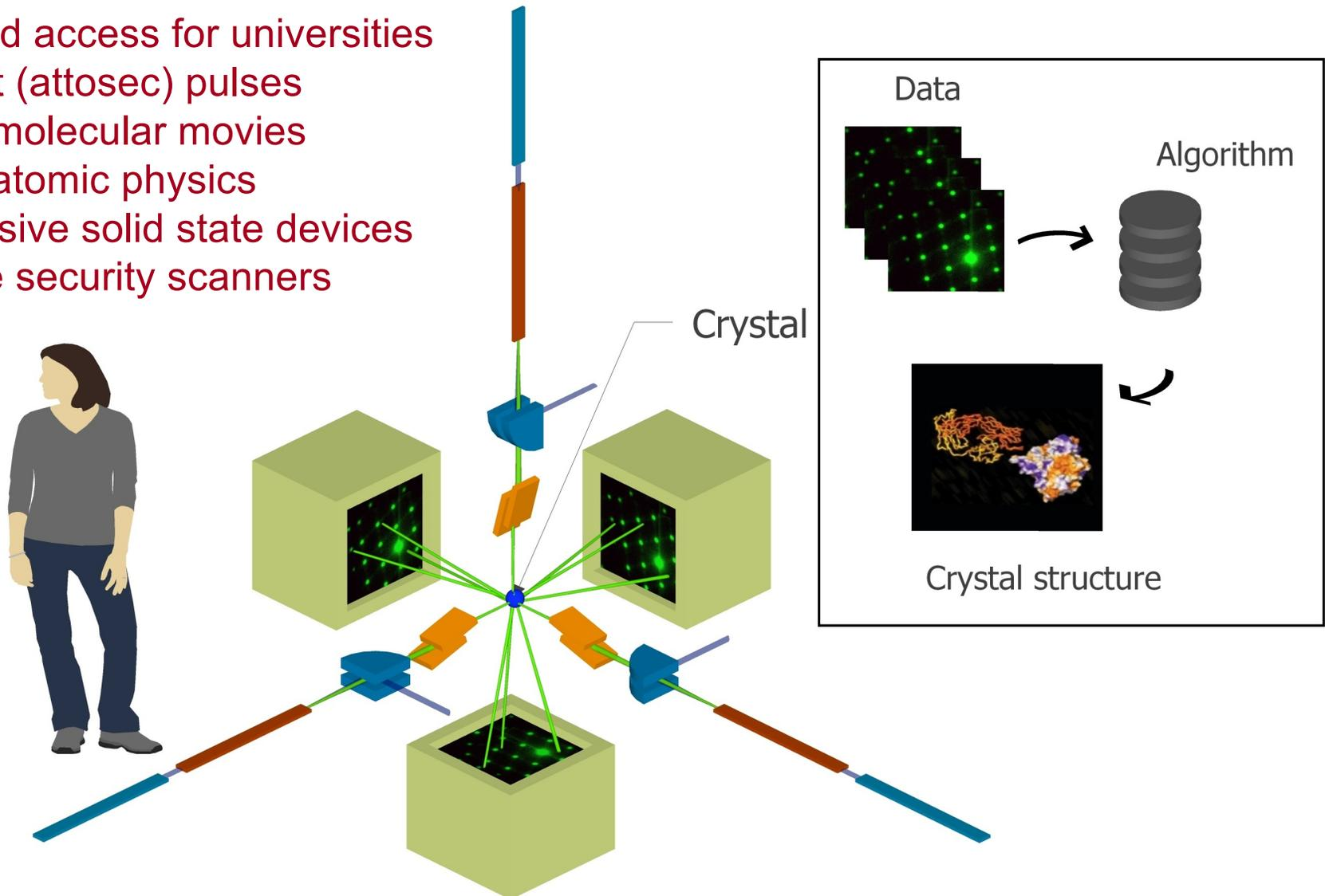
Concept for multi-axis ultrafast tomography with DLA based XFELs (K. Wootton)
