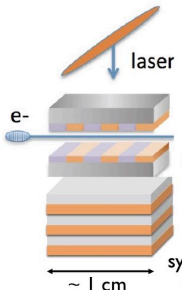
One potential use for a dielectric deflecting structure is as a miniature (~1cm total undulator length) EUV light source
