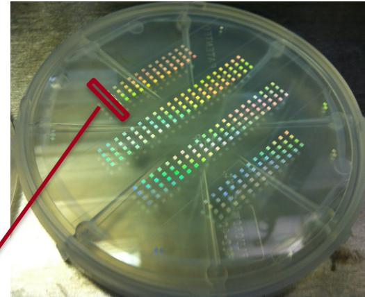
bonded silica phase reset accelerator prototypes fabricated at SLAC/Stanford
