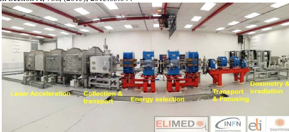
Figure 1: Photo of the ELIMAIA accelerator section (left) and of the ELIMED beam transport (collection, energy selection, transport and focusing and dosimetry) in November 2018, just after the installation in the RP3 hall at ELI-Beamlines (CZ)
