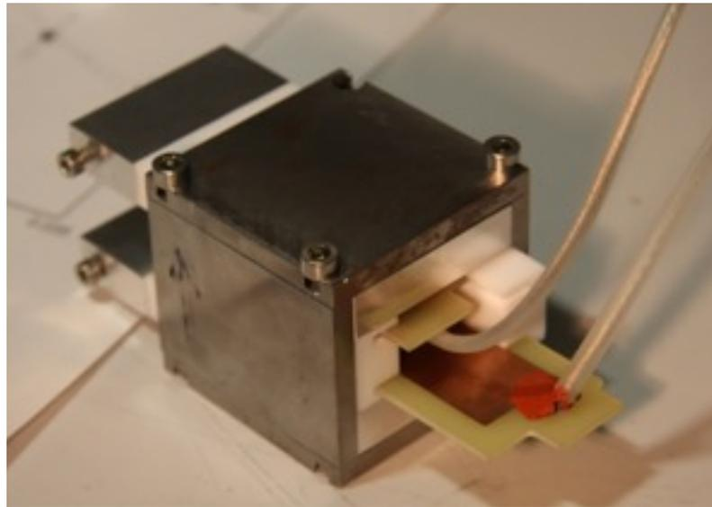
The main proton/ion diagnostic in LOA: MCP/TP
