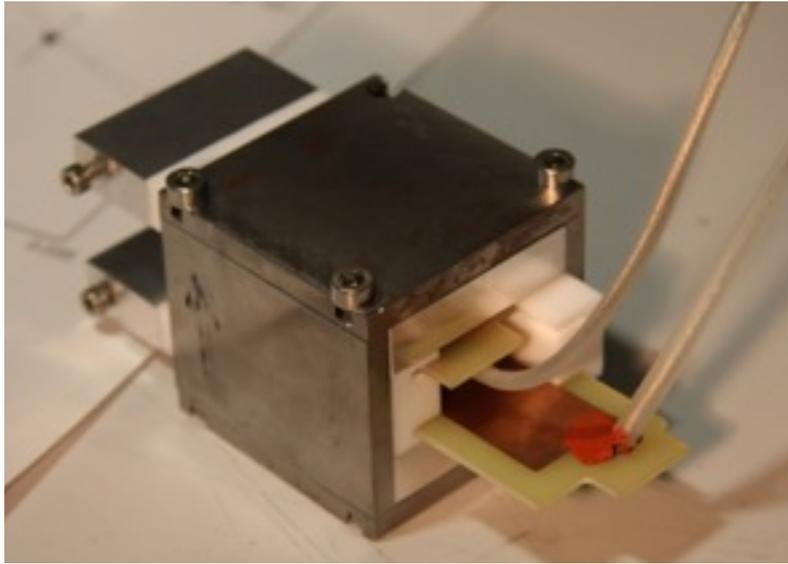
The main proton/ion diagnostic in LOA: MCP/TP
