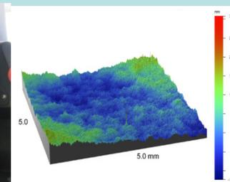
Figure 10. A high resolution scan of the surface of a microscope cover slip
