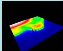
Figure 3. CMM laser probe surface scan of part of a 1p coin, (Blue to white range 150µm)
