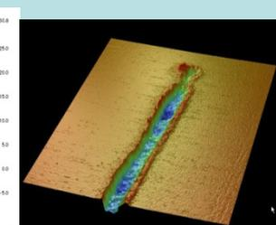
Figure 11. A high resolution scan of a laser etched groove
