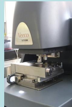
Figure 9. The Wyko NT9300 Interferometer
