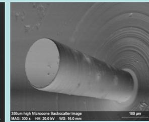
Figure 8. A backscatter SEM image of a hand turned micro-cone, showing machining marks and contamination
