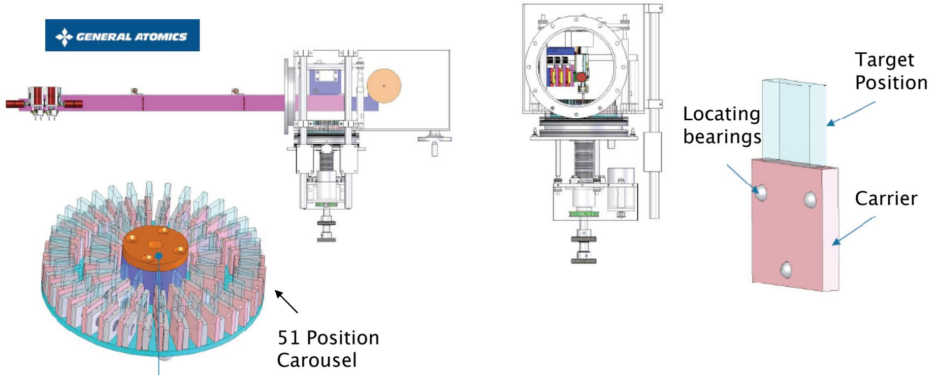
Telescopic cable reel arm with gripper to position target holder. Targets stored and picked from a carousel with 51 positions.
