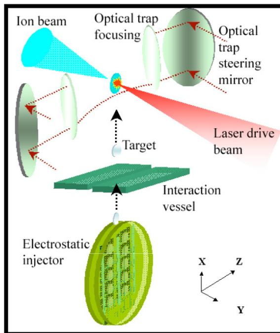
Original design concept for target delivery, optical trapping and target irradiation to produce ion-beams
