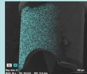
Figure 7. A elemental map showing an Aluminium tube around an AFI cone
