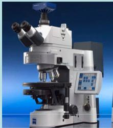
Figure 1. An AxioImager Microscope
