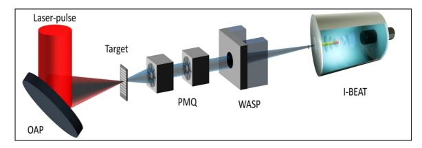
Figure 1: Schematic drawing of the I-BEAT integrated in a beamline for laser accelerated ions. The laser pulse is focused via an off-axis parabolic mirror (OAP) onto a target, from which the ions are accelerated. Two permanent magnet (PMQ) are installed to focus the ions and and a wide angle spectrometer (WASP) filters out electrons and low energy particles. The ionoacoustic signal of the particles in the I-BEAT detector is recorded with a transducer (visible in black).
