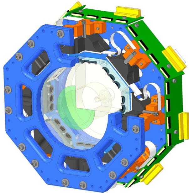
*Figure 1: Design of the new online detector for angularly resolved reconstruction of proton energy spectra based on scintillator emission tomography.*
