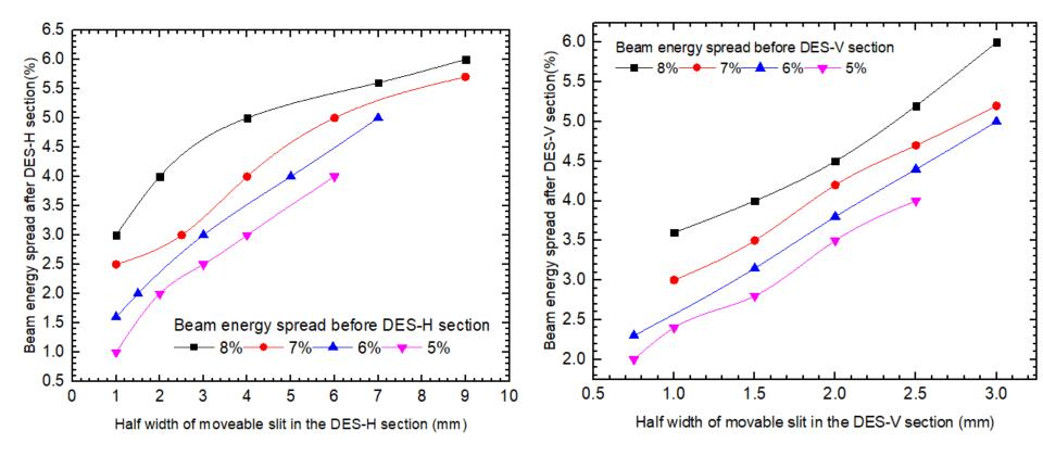
The moveable slit set between DES section remove particles with energy deviation and neutral stray particles produced by laser acceleration.
