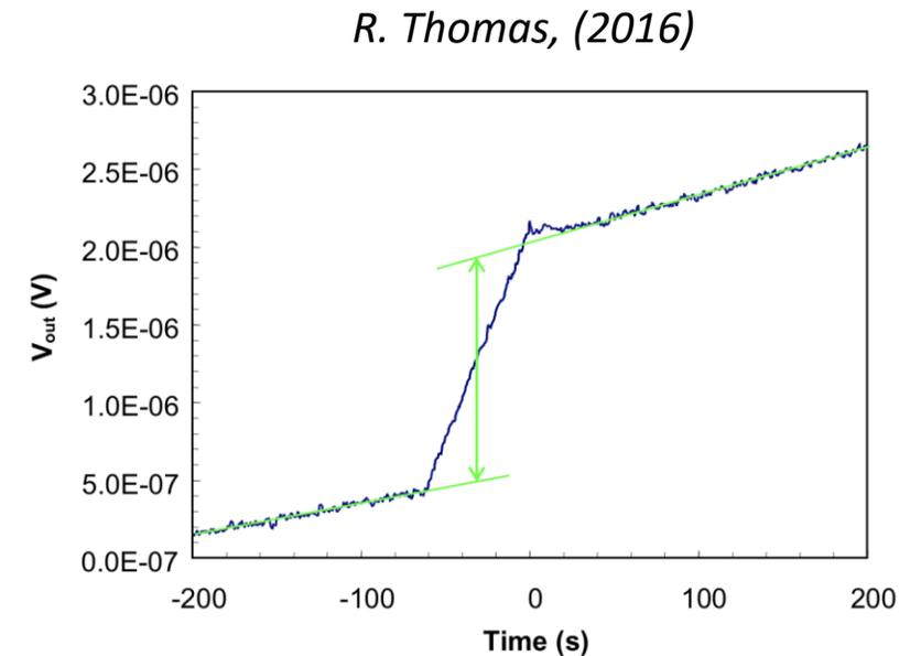
**Primary standard for absorbed dose measurements in clinical proton beams based on graphite calorimeter at NPL**
