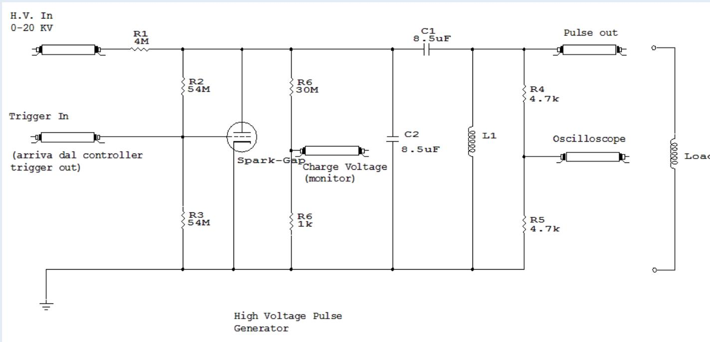
Basic scheme of the foreseen pulsed high voltage power supply.
