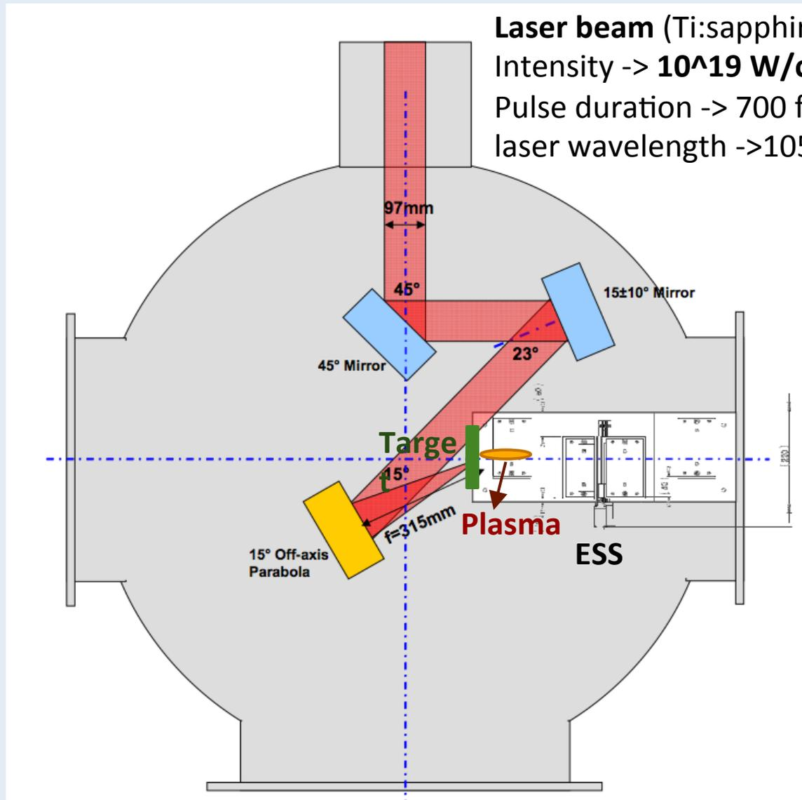
**Laser beam** (Ti:sapphire-Nd:glass)
