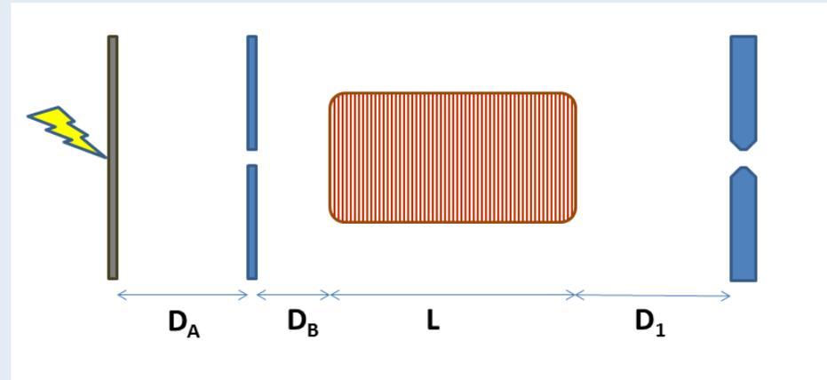
FIG. 4: Schematic draw of the transport line.  $D_A = D_B = 10$  mm,  $D_1 = 510$  mm,  $L = 300$  mm, first iris radius = 0.5 mm, second iris radius = 0.6 mm, second iris minimum thickness = 5 mm.
