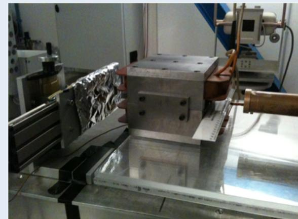
THOMSON SPECTROMETER: Analysis of proton and carbon beams ( $Q=+1$  to  $+6$ ) from 0.1 MeV to 10 MeV
