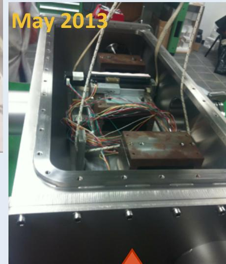
The ESS inside its vacuum chamber
