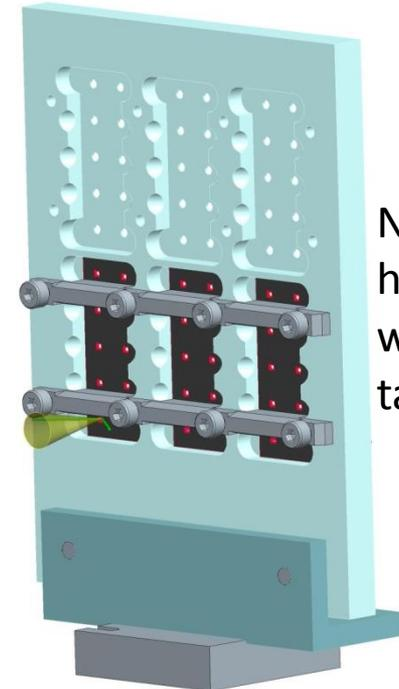
Novel target holder design with separated target support
